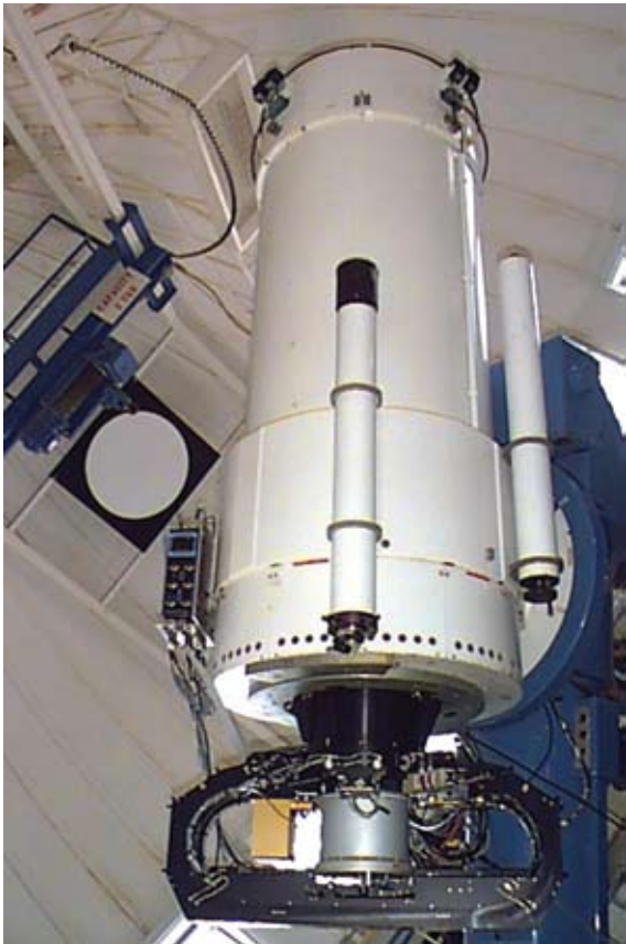
The Mosaic wide field optical imager, attached to the 0.9-meter telescope at Kitt Peak National Observatory, is one example of technology being used to extend our senses.
